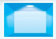
A simplified light distribution below the light tunnel's diffuser in the middle of the room without windows.
