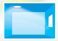
Depending on the user's requirements, colour of walls (possible diffusion and reflection of the light) and furniture placement - this is a basic scheme for light tunnel location in a room with a window. With two different sources of daylight, corner areas are not of great importance in this configuration and are pretty well illuminated. The placement of a light tunnel too close to a wall opposite to a window may diminish the overall light in the middle zone.
