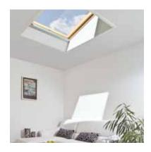
Modern building with a flat roof is becoming more common view. In this kind of roofs, using special system, we can install roof windows in an easy way. Such solution lets natural light and fresh air inside the room. The window can be operated by remote control.
