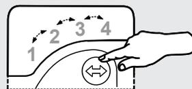
**2** Within 1,5 sec. press once IN/EX button and once button of movement of a given group to which device is to be added. LEDs 1,2,3 will light up.
