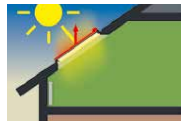
The external accessories keep the sun's rays outside the pane, reduce the heat flow and help prevent the room from overheating.
